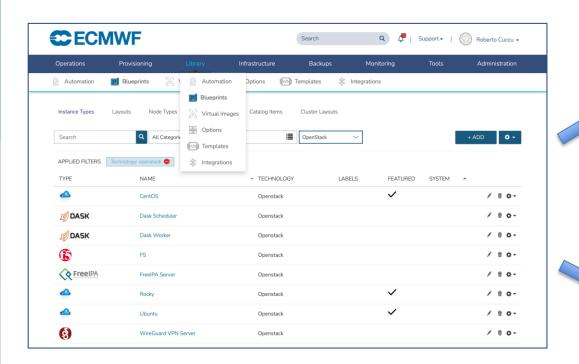
Blueprints feature together with automation tools allow the setup of reproducible application environment for their flexible on-demand deployment.
