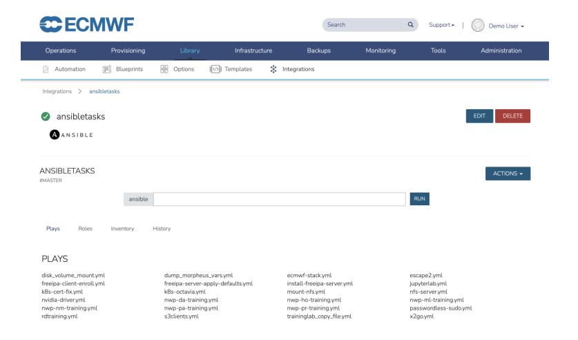
**Automation Integrations** can be added to enable the use of configuration management tools, e.g. Ansible
